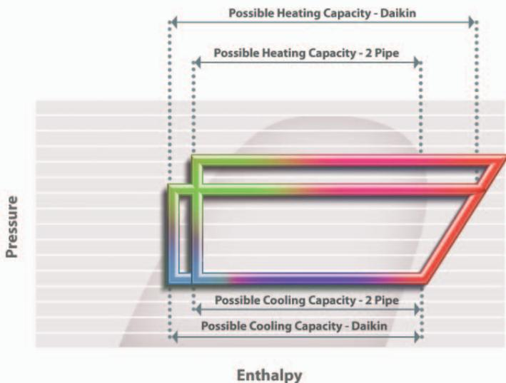
These charts describe the difference between two systems. One shows a system with significantly more heating capacity available when in heat recovery mode. The other shows the extra power needed to reach the required system condensing temperature. Charts represent theoretical operation in cooling dominant heat recovery mode.
