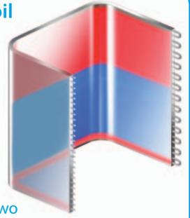
This provides 50% more surface area across which heat can be exchanged, so the compressor needs less power.
