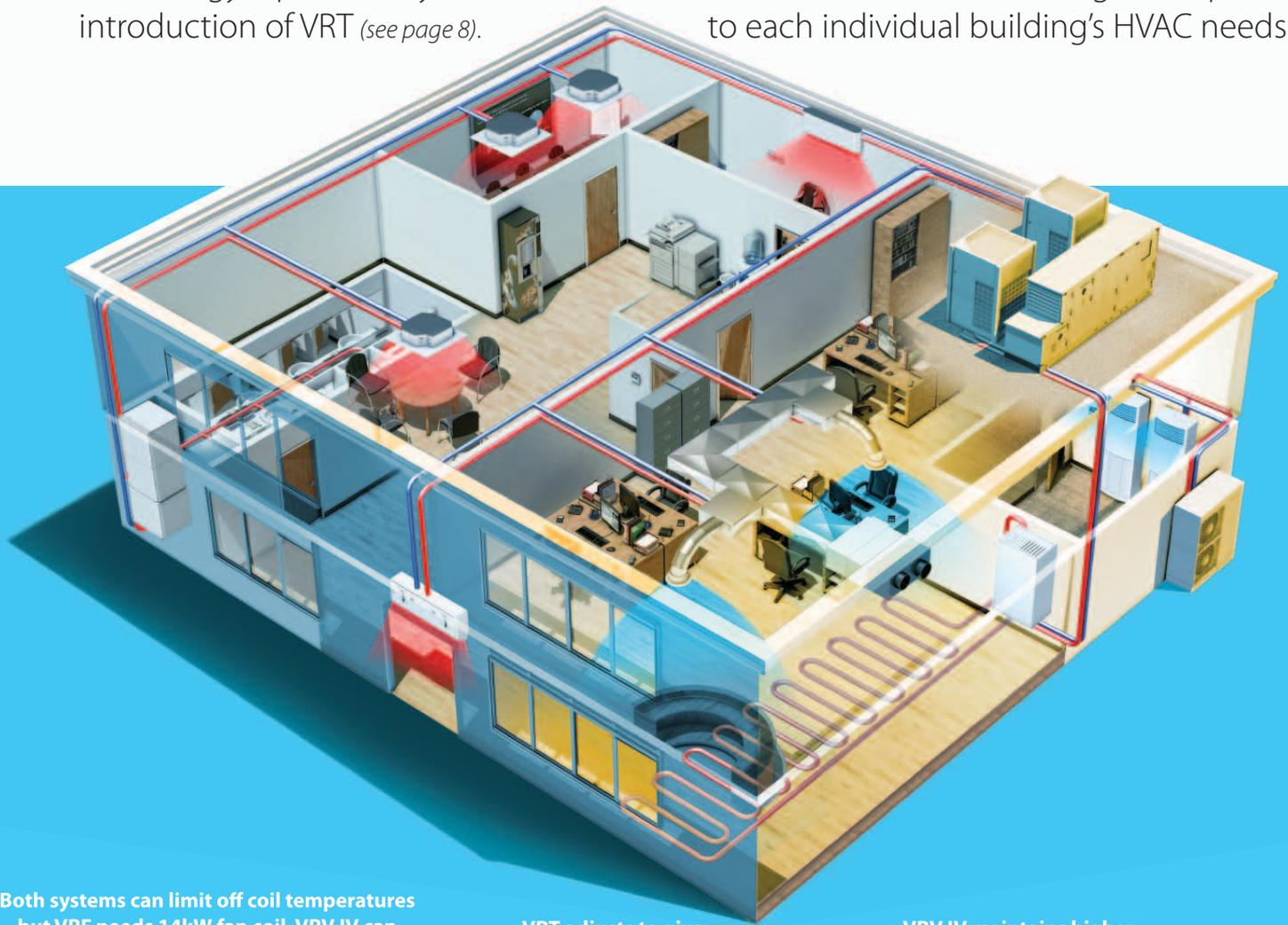
Both systems can limit off coil temperatures but VRF needs 14kW fan coil. VRV IV can do same job with 8kW fan coil – and can switch more capacity to meet load.
